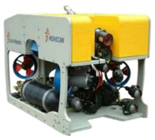
system, or a 6 station general function valve pack and HPU, enabling the use of a range of manipulators and hydraulic tooling.
